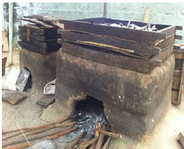
Figure 1: A single unit Chorkor smoker with 3 smoking trays on top (photo from Owusu et al., 2019)
