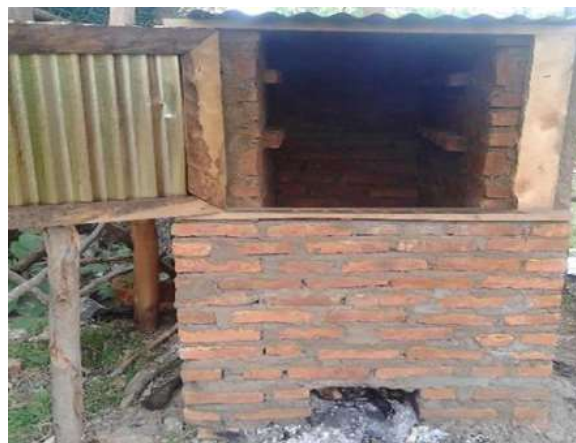
Figure 3: Front view of Altona oven in Ethiopia constructed of brick (photo from Hailu et al., 2019)
