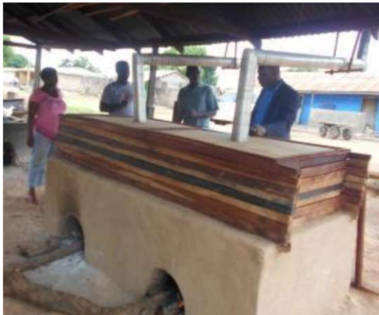
Figure 2: A running Morrison oven with approximately 7 trays. The two metal chimneys above each stokehole allow for people to comfortably stand around the smoker while operating (photo from Pemberton-Pigott et al., 2016).
